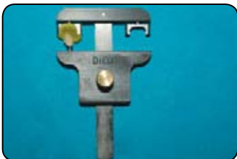
Seating jig fabrication
